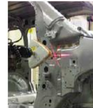
The Nikon Metrology XC65D laser scanner captures geometric features from 3 sides simultaneously.
