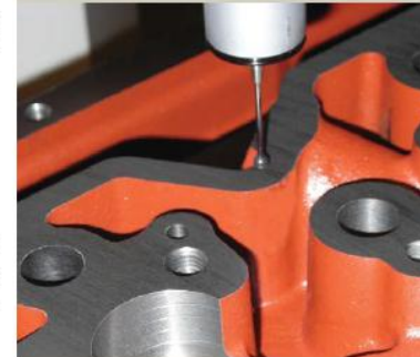
Cummins runs many touch sensor inspection tasks, including the scanning of surface valve cover sealing.
