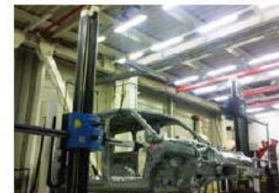
Ford Otosan successfully made the shift to the XC65D laser scanner for automobile vehicle body inspection.
