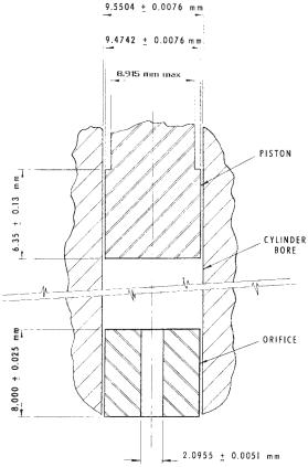
FIG. 2 Details of Extrusion Plastometer
