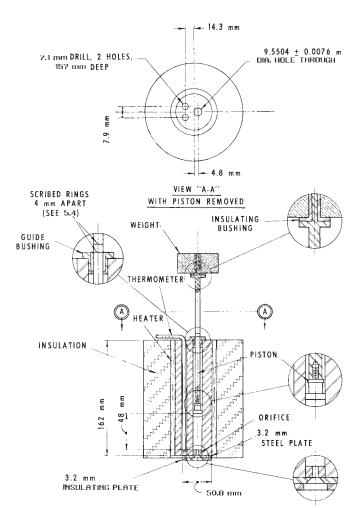
FIG. 1 General Arrangement of Extrusion Plastometer
