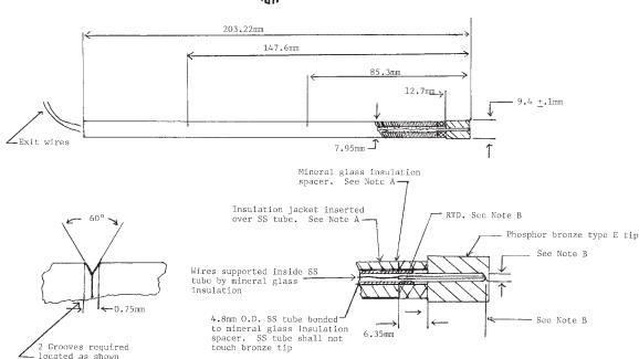
FIG. 3 Example of a Temperature Calibration Device
